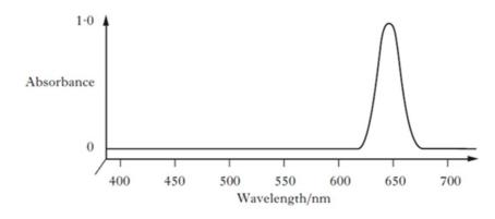
The absorption spectrum of a solution of sodium tetrachlorocobaltate(II) is shown above.
