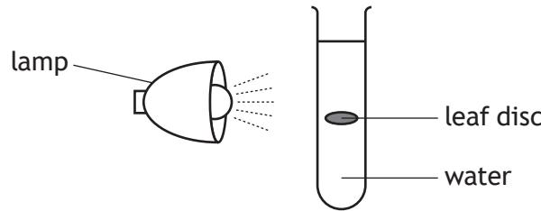
After the lamp was switched on, the time taken for the leaf disc to float to the surface was recorded.
